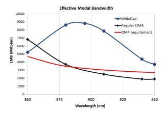
The capacity can be further increased by implementing advanced modulation formats such as PAM-4. In the laboratory, a 180Gbps transmission over a WideBand MMF with four 45Gbps PAM-4 WDM signals was successfully realized, the BER of which had a range of over 300 m, while a maximum of 150 m was achieved with OM4-MMF. These results show the performance data of WideBand MMFs to realize 40, 100 or 200Gbps without the need for parallel fiber optic infrastructures.
