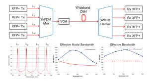
In order to guarantee a constant effective bandwidth of 2,000 MHz \* km, the EMB must be 4.700 MHz \* km at 850 nm and must not be less than 2.700 MHz \* km up to 950 nm (see FIG. 2). WideBand MMFs that meet these specifications are made by optimizing the core profile and tuning the alpha parameter in the GI core glass to shift the peak EMB to 880 nm.
