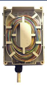
The Verticasa Storage Box is used to coil and store over-lengths of Verticasa fibre modules. The box can be used at the top of a vertical riser cable or on the end of a horizontal cable run. The box has a single cable entry for cables of up to 15mm in diameter. The box can be supplied configured for either internal or external use and can accommodate up to 225 metres of 900 micron fibre modules.
